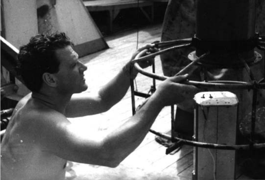
K. N. Fedorov (IOE Secretary, 1963–69) on board a research vessel in 1972, checking the CTD (Conductivity-Temperature-Depth) probe.
