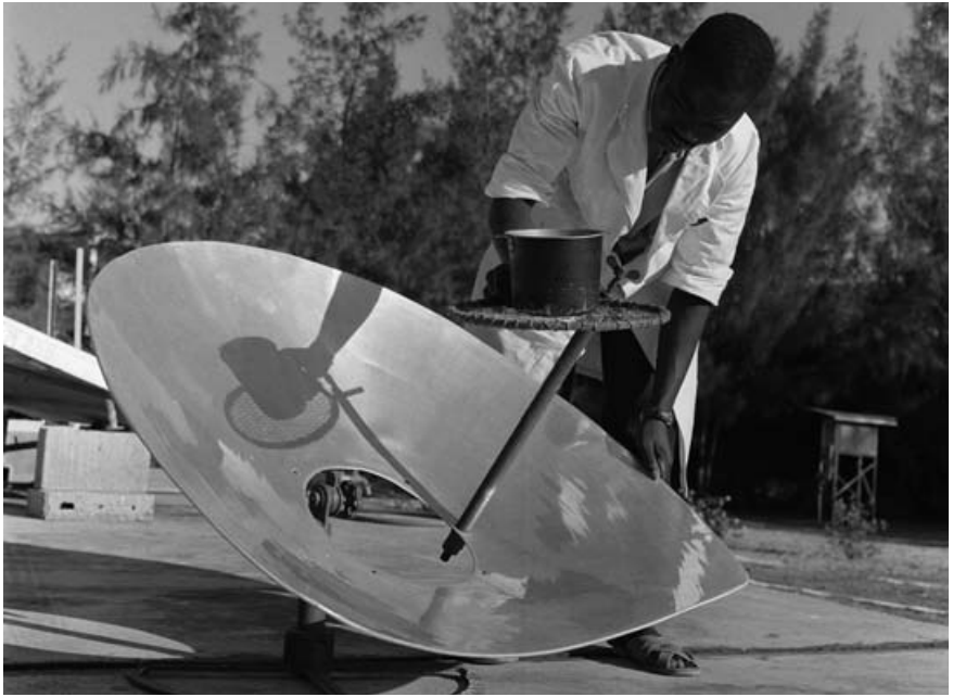
Solar oven at the UNESCO-assisted Solar Energy Laboratory of Dakar University, Senegal, 1962.
